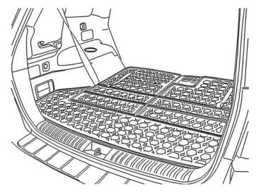
Place cargo tray in trunk area with the logo at the front of the vehicle with rear seats down as shown. Pull rear seat straps through cut-outs in tray. Ensure tray makes full contact with the trunk floor.
