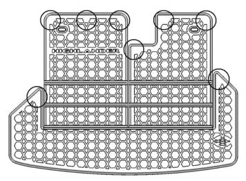
Rub/massage areas of cargo tray shown to ensure proper attachment to seatback before actuating rear seats up.
